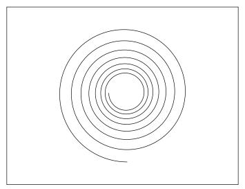
FIGURE 3-4 Undriven pendulum phase space: "point attractor."
