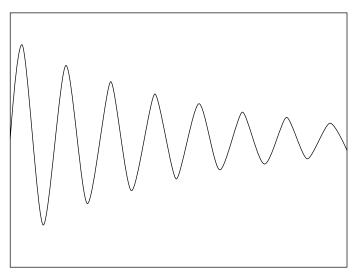
FIGURE 3-3 Undriven pendulum time series.
